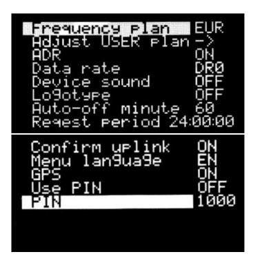
Frequency plan – choice of the frequency standard. EUR – European frequency plan. RUS – Russian frequency plan. USER – custom frequency plan.
